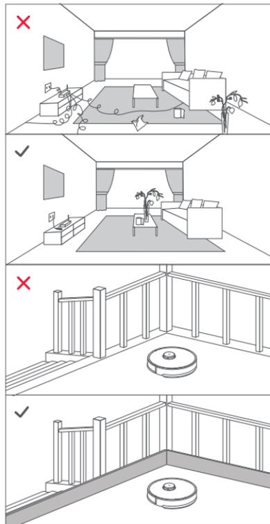
1. Tidy cables and loose items from the ground and move any unstable, fragile, precious, or dangerous items to prevent personal injury or property damage due to items becoming tangled in, struck by, or knocked over by the robot.
