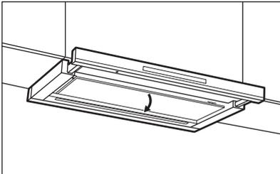
2. Pull the handle on the filter underneath the hood and slightly tilt the front of the filter down.
