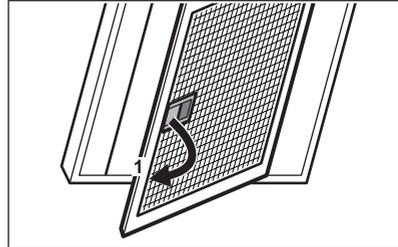
3. Clean the grease filters by hand using a sponge with non-abrasive detergents, or clean them in a dishwasher. We recommend cleaning the grease filters by hand.
